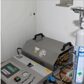
JBL CO2 Refill Service Refill service for the filling of JBL CO2 cylinders
